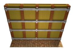
**4.** Fix the ReductoClips on the bottom of the timber joists in the appropriate positions.
